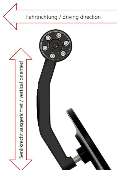
7) Tighten screws (C1) and (C2) max. 3Nm after you adjusted the mirror stem and mirror head correctly.
